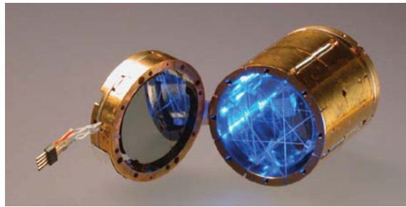
Figure: A 46 g BGO bolometer (right) shown separately with the Ge disk used as optical detector (left).
