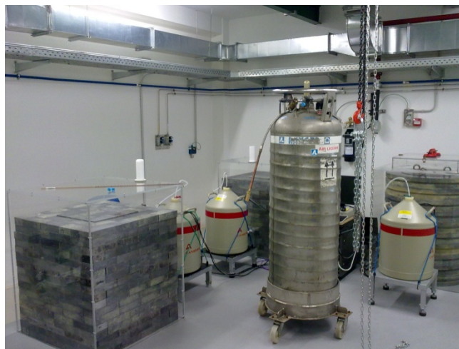
The three Hyper Pure Ge counters, hidden in their Pb+Cu shields, are shown in the figure
